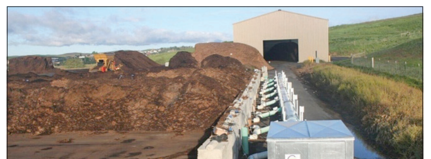
Figure 8. Aerated static pile. Photo: Washington State University
