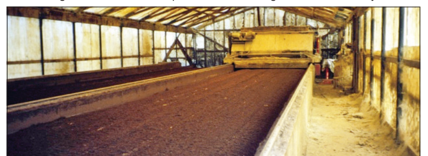
Figure 9. Agitated bay or channel. Example shown composting chicken manure in a glasshouse. Photo: Washington State University
