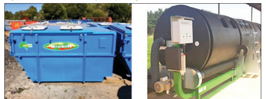
Figure 7. Examples of containerised composting systems, with the BiobiN and the Ecodrum.
