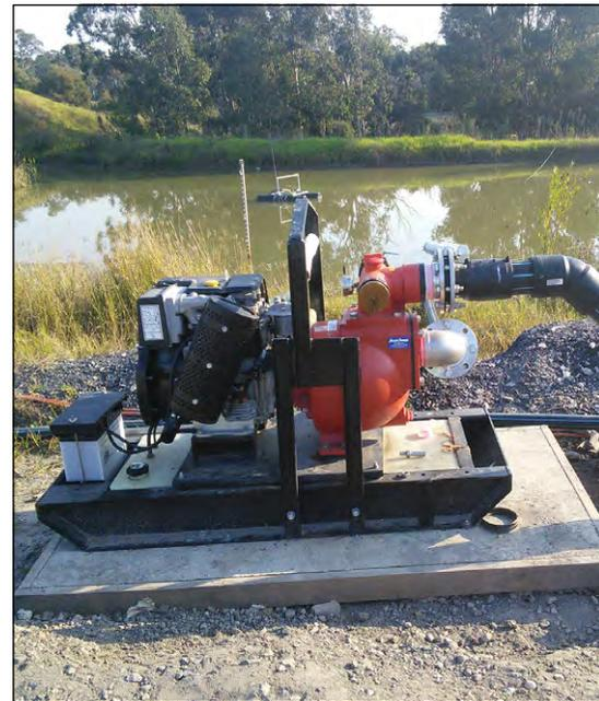
Veolia's timber recycling facility at Horsley Park is protected from spontaneous combustion by an Aussie self-priming four-inch diesel drive high pressure pump.
