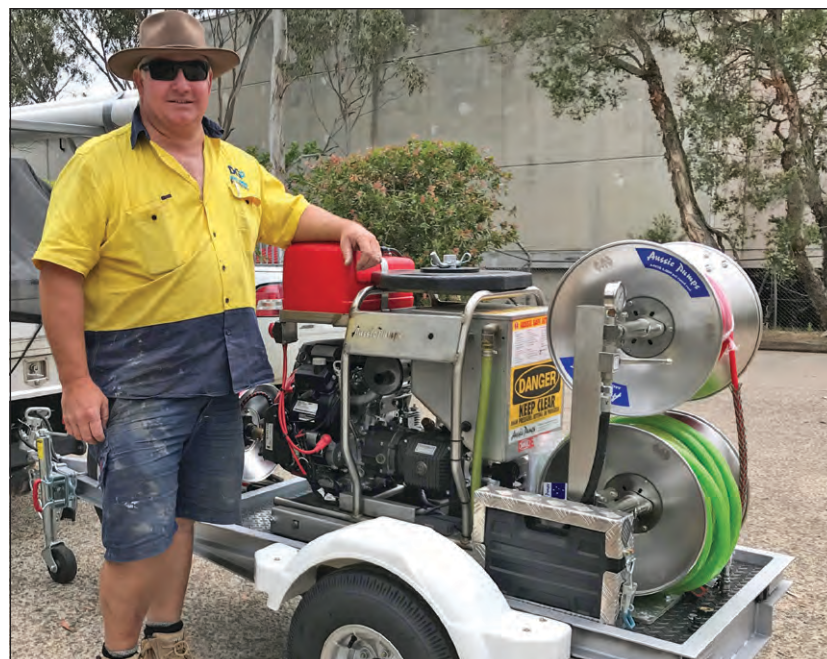
Making it easy to get jetting, Aussie Pumps new compact trailer-mounted jetter for efficient drain cleaning and wash down.
